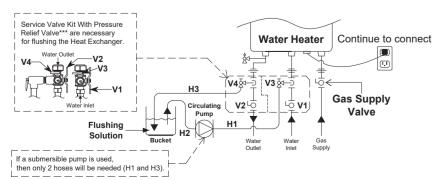
\*\*\* Service Valve Kit With Pressure Relief Valve may be purchased as an accessory from an authorized wholesaler They allow for full diagnostic testing and easy flushing of the system.
