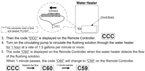
Please check whether the reverse connection of the hose (H1) and (H3) if the display number will not change In that case, the flow rate of the flushing solution may be under 1.5 gallons per minute.
